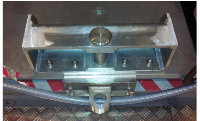
Fig xx: Rope anchor feature would clash when moving offline but is temporarily removable
