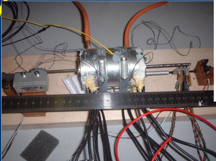
**New stator (24 coil design).**
