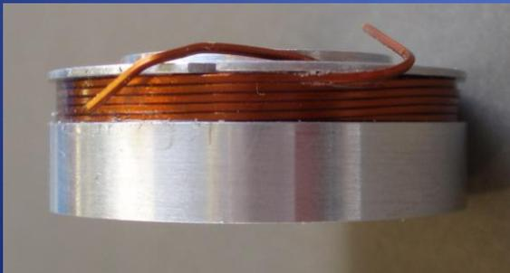
Coil Wound using Square Wire. Design changed to improve the coils magnetic symmetry/reproducibility.
