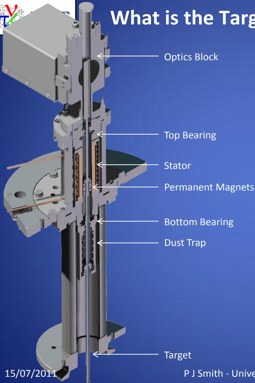
The target mechanism is an electromechanical device that rapidly inserts a small titanium target into the circulating proton beam of ISIS immediately prior to extraction without unduly disturbing the primary proton beam.
